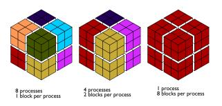
Figure 2: Allocation of eight blocks to processors. Blocks are colored by the process to which they belong.
