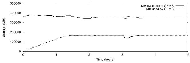
Fig. 3. System Reponse to Induced Server Faults.
