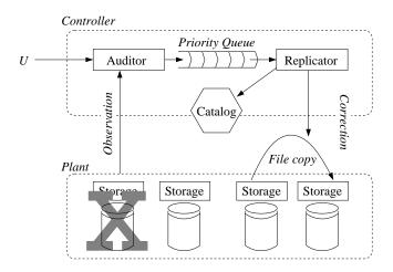
Fig. 2. Replica Control Loop.
