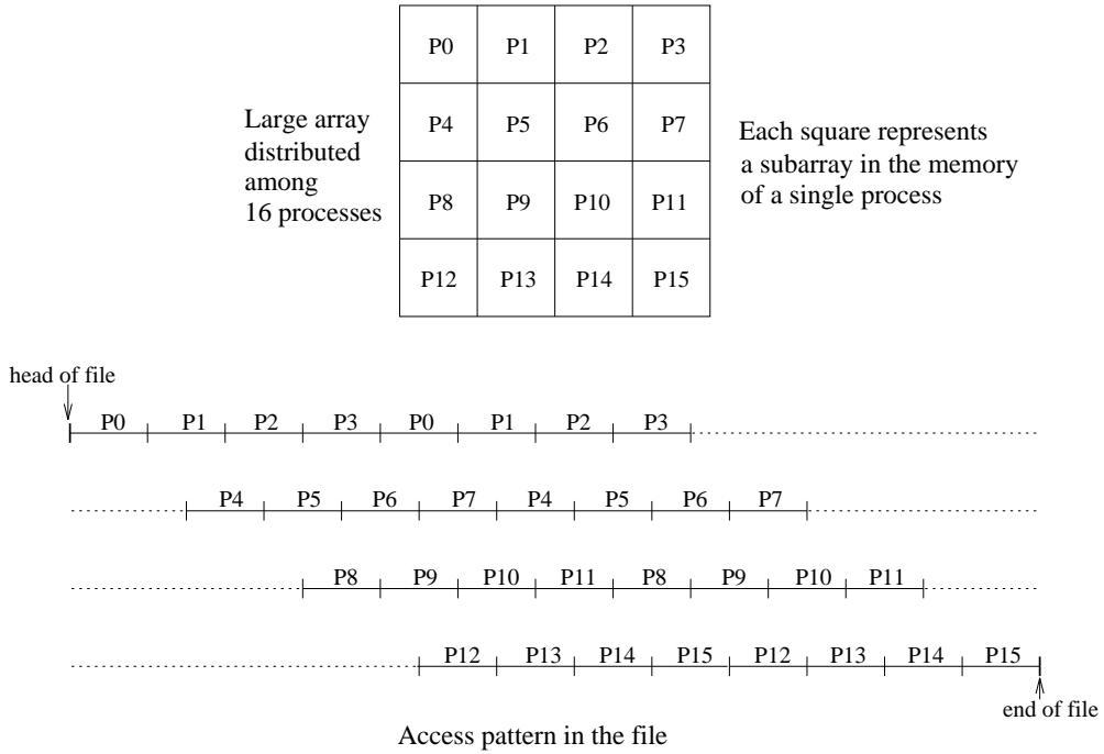
Figure 1: Distributed-array access
