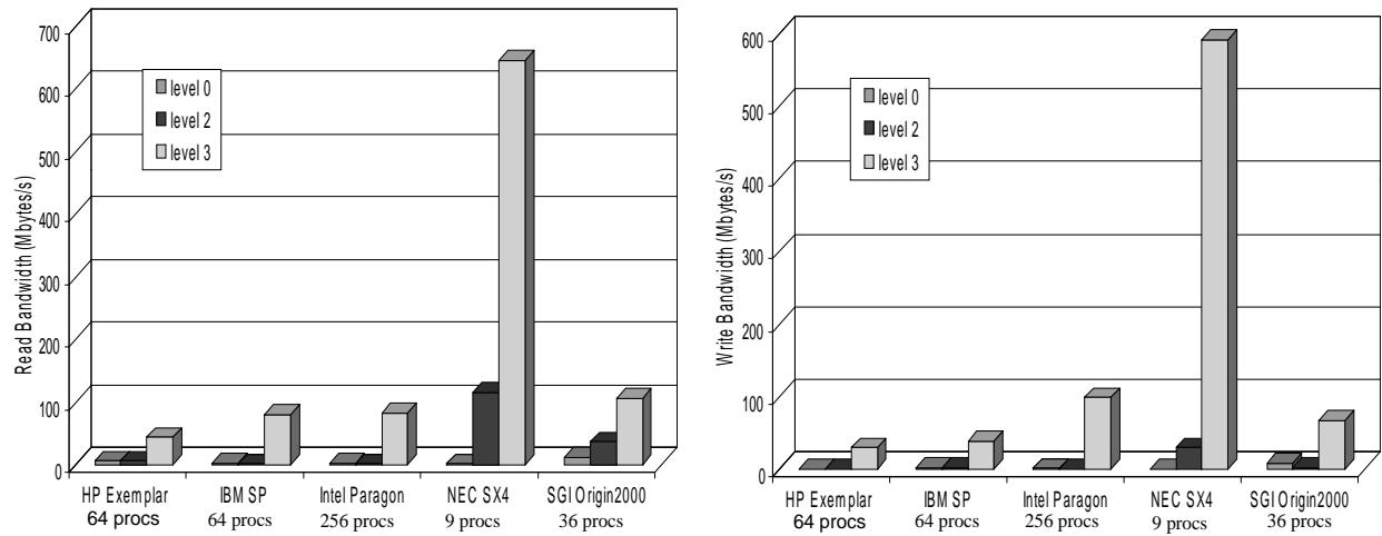
Figure 11: Performance of BTIO (Class C, problem size  $5 \times 162 \times 162 \times 162$  double precision  $\approx 162$  Mbytes). Level-1 results are not shown because, for this access pattern, ROMIO simply translates level-1 requests internally into level-0 requests.
