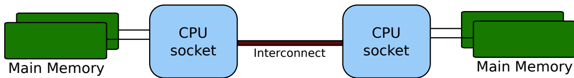
Figure 23: Schematic of a two-socket NUMA system. Processes should be spread across both CPUs to obtain full bandwidth.
