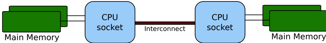
Fig. 3.2: Schematic of a two-socket NUMA system. Processes should be spread across both CPUs to obtain full bandwidth.
