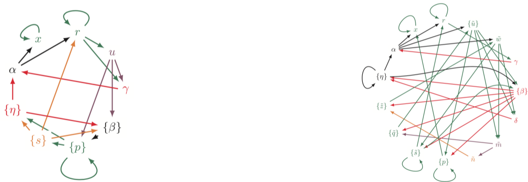
Figure: Schematics of the main loop of the Flexible Conjugate Gradient (FCG; left) and the Modified Pipelined Flexible Conjugate Gradient (PIPEFCG; right) methods. Data dependencies in FCG preclude overlapping reductions with the application of the operator or the preconditioner. At the price of increased local work and storage, PIPEFCG reductions can overlap operator and preconditioner application.
