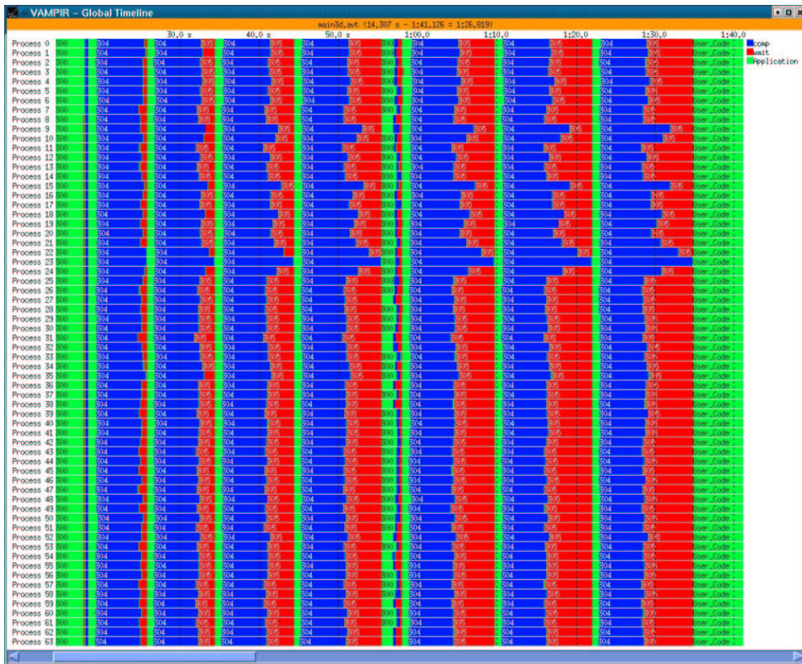
Figure 2 – VAMPIR Trace analysis on 64 processors
